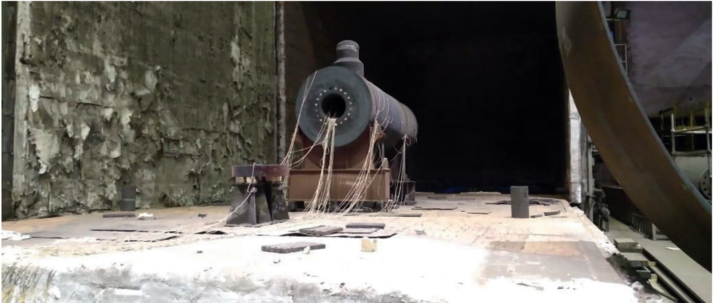
Figure 6. Thermocouples were installed at internal and external surfaces prior to furnace PWHT.
