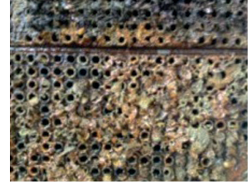
Figure 5. Biological fouling (algae and microbial slimes).
