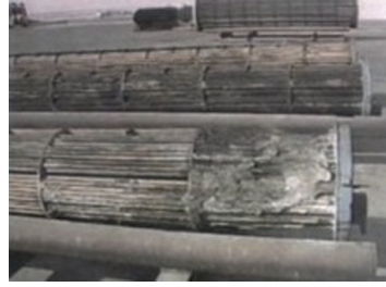
Figure 3. Fouling accumulation on shell side.
