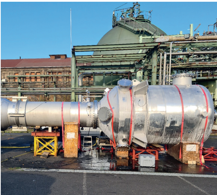
➤ Acoustic Emission Testing: Sensors on a process vessel.
