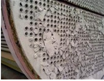
Figure 2. Clogged tubes by severe fouling.
