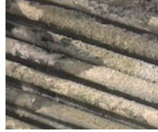
Figure 4. Under deposit corrosion.
