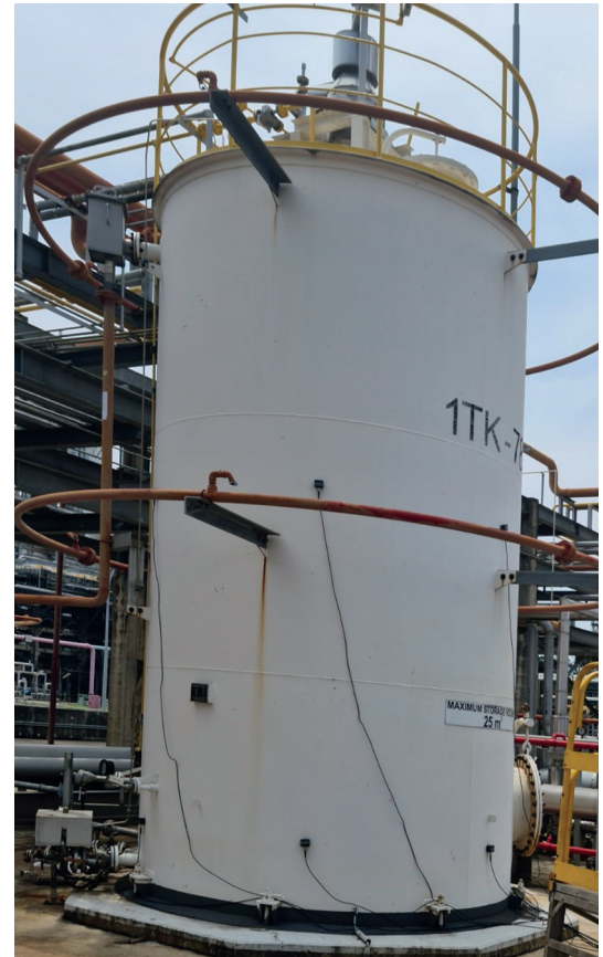
➤ A flat-bottom storage tank is inspected using Acoustic Emission Testing.
